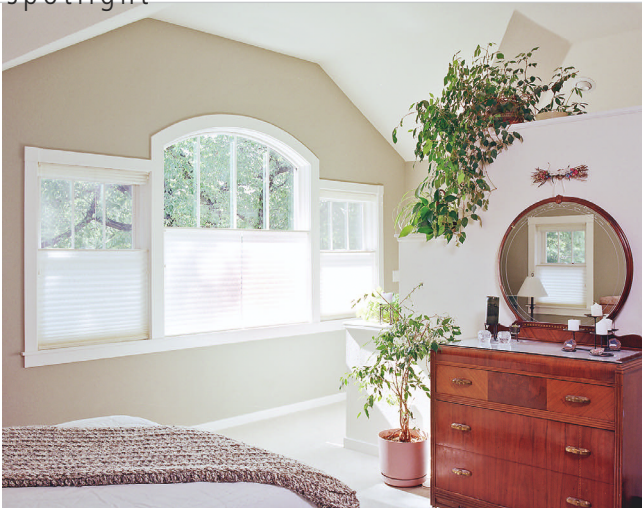
In the master bedroom, low-E windows with accordion blinds allow light and views but cut glare and heat gain. A glass-block wall at the head of the stairs, behind the bedroom's partial wall, draws in natural light, illuminating the stairwell. Photo by Fotoimagery.com
